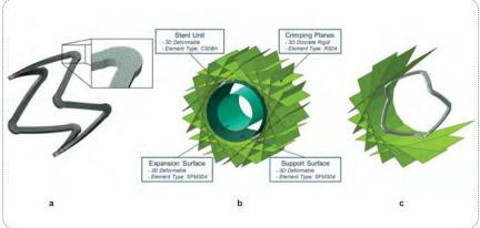
A finite element analysis was performed by studying an ideal stent unit (Fig. 1.a) with geometrical dimensions comparable with those of coronary stents. The stent unit was made of an elastic-plastic material whose plastic behavior was implemented according to Johnson-Cook plasticity model to reproduce PLLA performance. Two numerical simulations were carried out using ABAQUS® / Dynamic Implicit, each one made of five steps to properly reproduce the surgical stenting procedure (Fig. 2).
